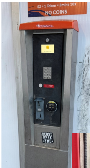
Istobal Self Serve units with coins, Nayax and keypad /push button select. These units have very small LED screens.
