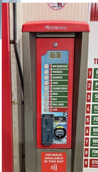
Facelift Istobal Self Serve unit with Nayax cashless, code scanner, speaker and 10.1" LED Touchscreen
